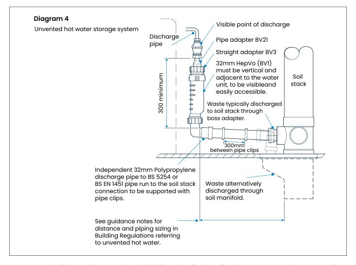
**Note:** Where the discharge pipe up to the tundish is 15mm the discharge from the HepVo trap to the SVP can be in 22mm metal pipework providing the discharge from the tundish does not exceed 8.2m in length.
