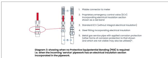
\* Note: The applied corrosion protection outer sleeve on a metal service pipe should not be considered as a means of providing the electrical insulation.
