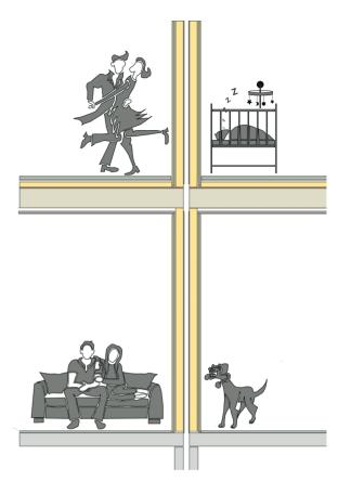
New homes are designed and built to better standards with mandatory measures to minimise noise transfer between adjacent homes through walls and floors.
