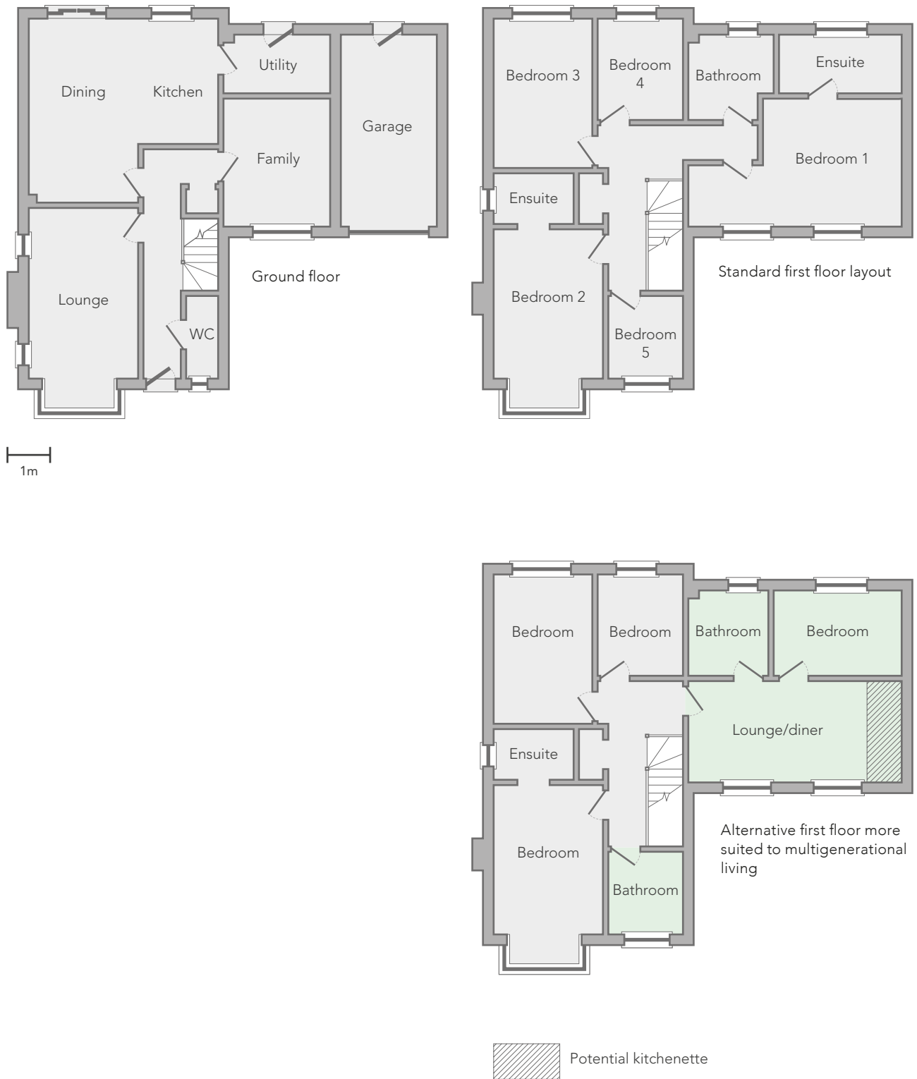
Figure 13 A house plan that, with some redesign of the first floor, could provide greater flexibility for multigenerational living – in this case providing a self-contained suite as an alternative to a large master bedroom. See notes to Figure 12.
