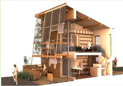
Hanham Hall, Bristol. All living spaces face south and have high ceilings and large windows
