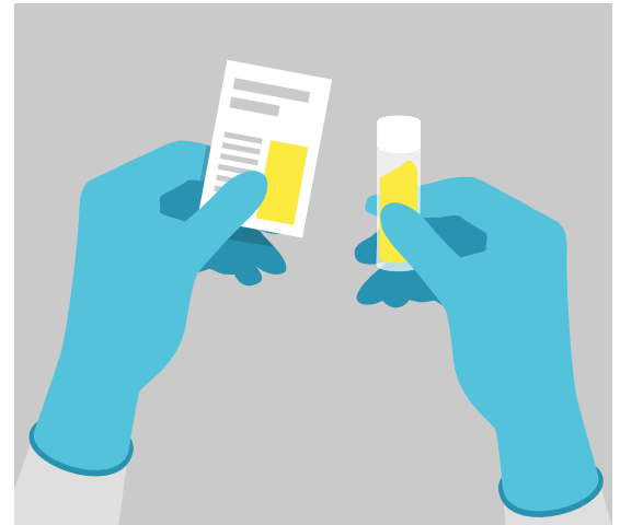
5.2 A water sample is taken and colour tested for the right concentration of inhibitor
