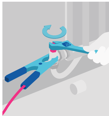
5.4 Lockshield valve adjustment
