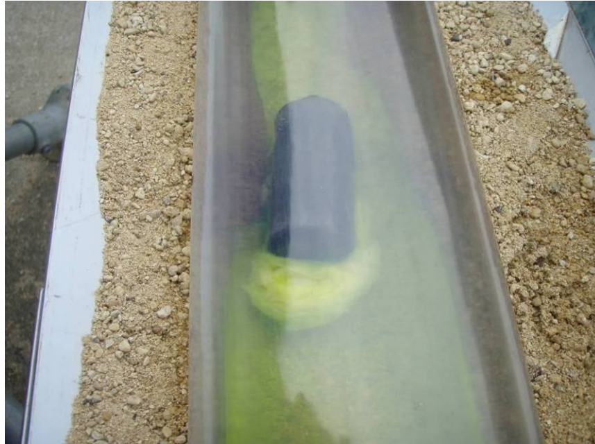
Photograph 11.1 Paper offset with water escaping past one side of the solid
