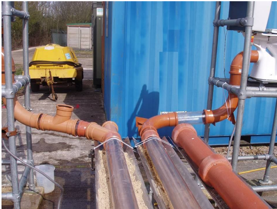
Photograph 6.2 Test rig – Typical arrangement (left) and long radius bend arrangement (right)
