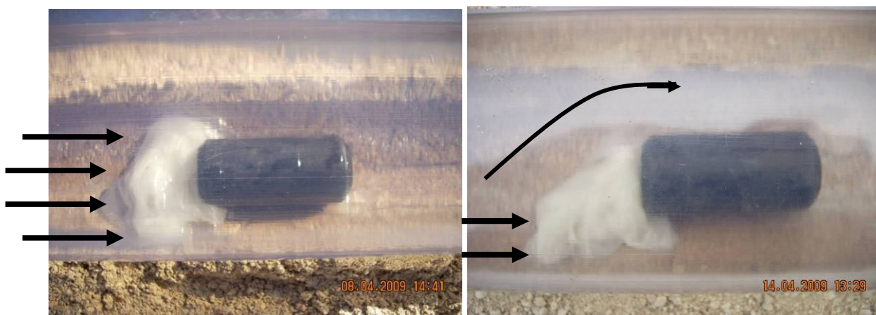
Photograph 5.1 Positions of paper behind the solid – Complete dam (on the left) and gathered on one side (on the right)
