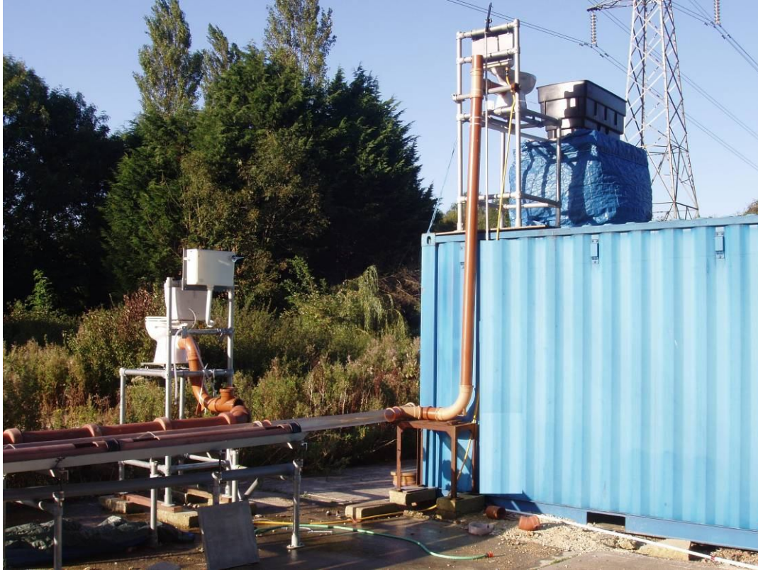
Photograph 4.5 Upstairs WC and bath soil stack arrangement
