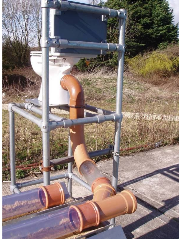
Photograph 4.3 Test facility – Typical inlet connection to the drainage system
