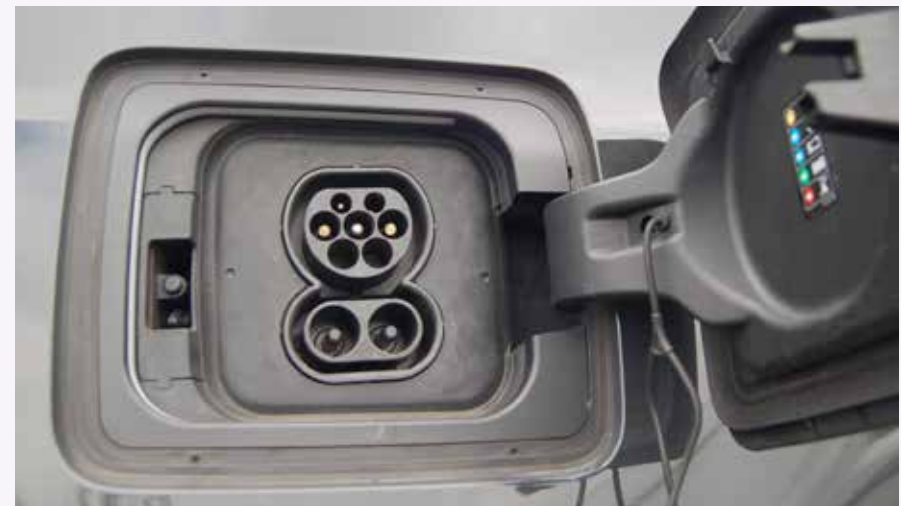
Figure 3 Type 2 (top) and CCS (bottom) sockets as typically fitted to EVs
